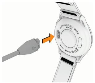
2 Plug the other end of the cable into a USB charging port. The watch displays the current battery charge level.
