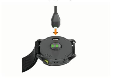
2 Plug the large end of the USB cable into a USB charging port. The watch displays the current battery charge level.
