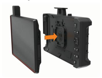
3 Press down the lock latch 1 completely and slide the lock switch 2 towards the latch.
