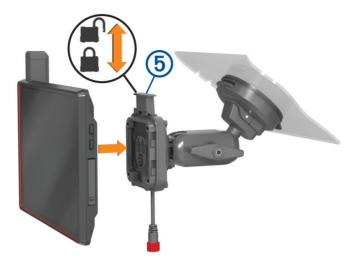
9 Push down the lock (5) to secure the device to the mount.
