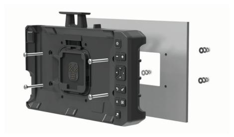
10 Secure the dock to the mounting surface using the appropriate hardware.
