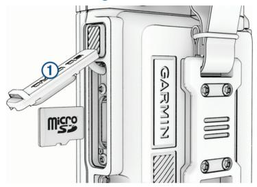
2 Insert the memory card with the gold contacts facing the front of the device.
