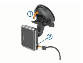
2 Plug the vehicle power cable 2 into the port on the mount.
