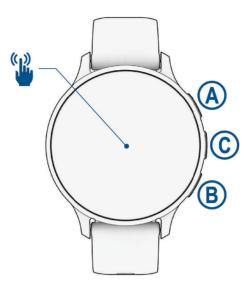
(A) Action button: Hold for 2 seconds to turn on the watch.
