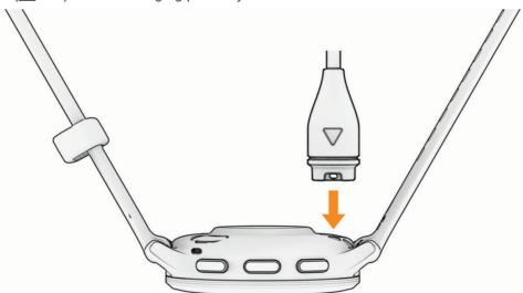
**2** Plug the other end of the cable into a USB charging port. The watch displays the current battery charge level.
