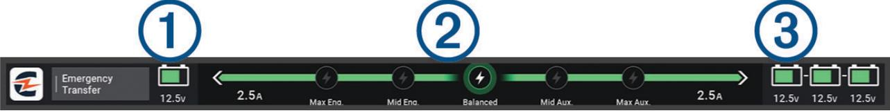
The screenshot shows a CHARGE layer interface with three numbered callouts: 1. Engine battery status (引擎電池狀態), 2. CHARGE priority order setting (CHARGE 優先順序設定), and 3. Auxiliary battery status (輔助電池狀態). The interface includes an Emergency Transfer button, a 12.5v battery icon, a 2.5A current indicator, and a central charging control bar with Max Eng., Mid Eng., Balanced, Mid Aux., and Max Aux. settings. On the right, there are three 12.5v battery icons.
