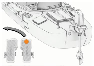
The nose of the propeller drive motor turns to the right, turning the kayak to the left.
