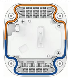
2 Gently lift the white tab to release the battery from the back cover.
