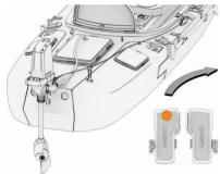
You can invert the right and left pedal response to emulate steering with a cable-controlled rudder instead (Inverting the Steering Response, page 35).
