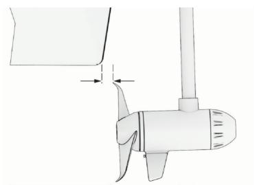
2 If necessary, adjust the motor depth to ensure sufficient space between the propeller and the hull (*Adjusting the Depth of the Trolling Motor*, page 4).
