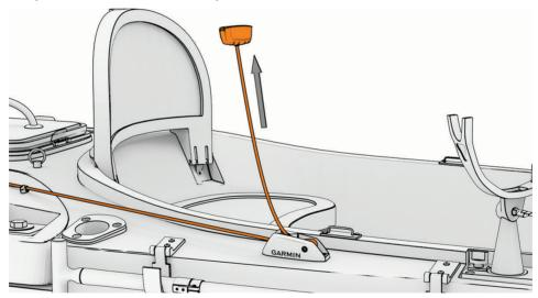
**2** Gently release the tension on the rope to lower the propeller drive motor into the water until it stops. The mount latch engages the locking pin, holding the motor in the deployed position.
