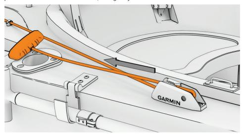
The rope is secure under tension in the cleat, holding the motor in the stowed position.
