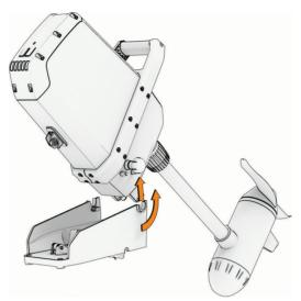
4 Lift the motor off of the mount using both hands.
