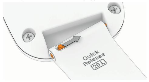
3 Align the spring bar with the other hole in the MOB tag, and release the pin.
