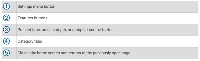
The categories tabs provide quick access to the main features of your chartplotter. For example, the Sonar tab displays the views and screens related to the sonar feature.
