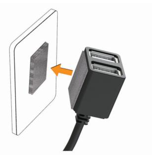
8 Connect the USB power cable from your Garmin Dash Cam device to a USB port on the Constant Power Cable device.
