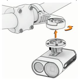
11 Adjust the headlight angle so it is parallel to the ground, and use the 4 mm hex key to tighten the screw.
