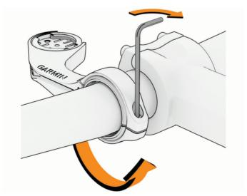
6 Install the Edge bike computer, and adjust the mount (optional).
