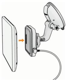
6 Plug the other end of the vehicle power cable into a power outlet in your vehicle.
