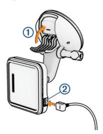
2 Plug the vehicle power cable into the port 2 on the mount.
