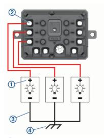
2 Connect the negative or ground wire 3 to an unpainted ground stud 4 on the vehicle frame, to a ground distribution block, or directly to the negative terminal on the battery.
