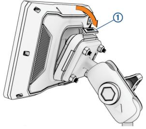
**2** Push the top of the device forward until it snaps into place.
