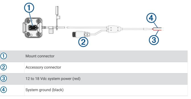
Additional parts are included with the device to cover different installation and wiring options. **Crimp Style Ring Terminals**: Connect the power supply wires directly to the battery terminal.
