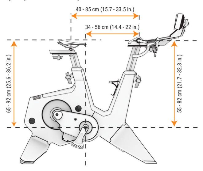
Before you assemble the Tacx NEO Bike Plus trainer, consider that the saddle and handlebar have set screws installed from the factory that can be adjusted and tightened using a hex key. To install the 4 handles, you must remove the 4 set screws using a hex key.
