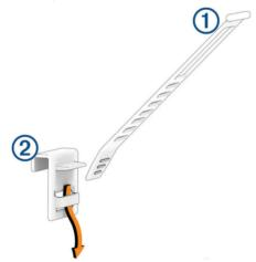
2 Connect the rubber strap to the back of the mount 3.
