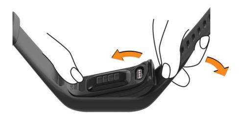
2 Insert the device into the band, and stretch the band material around the device. The mark on the device must align with the mark inside the band.
