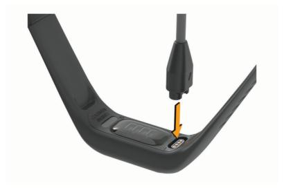
2 Plug the large end of the USB cable into a USB charging port. The watch displays the current battery charge level.
