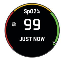
**NOTE:** If you are too active for the watch to determine your oxygen saturation, dashes appear instead of a percentage. You should remain stationary for up to 30 seconds while the watch reads your blood oxygen saturation.
