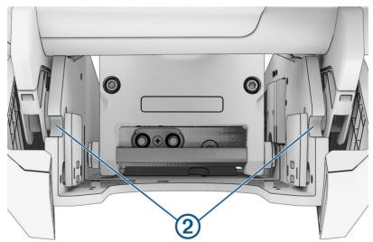
7 Apply a synthetic or marine grade, general-purpose grease to the latch receiver and both ramped surfaces and slots on the mount base so the locking mechanism slides smoothly into the receiver.
