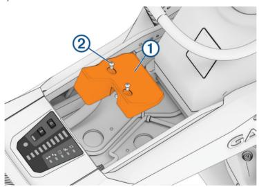
**TIP:** The molded collars on the cables should be in front of the servo landing pad when installed.
