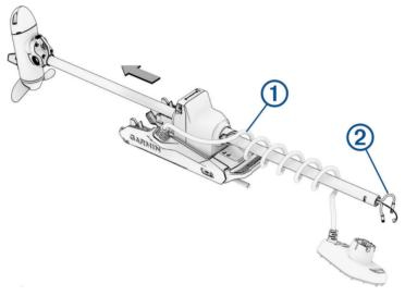
2 Slide the shaft and motor out of the steering servo, taking care not to damage the skeg and transducer or snag the cables or connectors ② as you pull it through.
