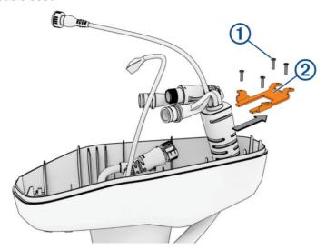
2 Pull the coil cable out of the shaft cap to remove it.
