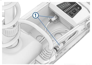
3 Tighten the locking collars to secure the cables.
