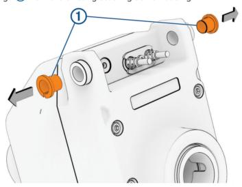
2 Clean all dirt and debris off of the bushings and out of the steering servo housing holes.
