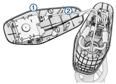
2 Release the latch 2 and pull the connectors apart to disconnect the motor data cable.
