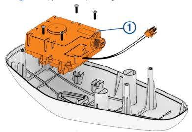
2 Using a # 1 Phillips bit or screwdriver, install the four screws that secure the antenna box to the upper shaft cap housing.
