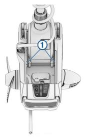
3 Apply a non-stick, dry-film lubricant to each hinge point, in the space between the moving parts 2, and allow it to dry according to the instructions provided with the product.
