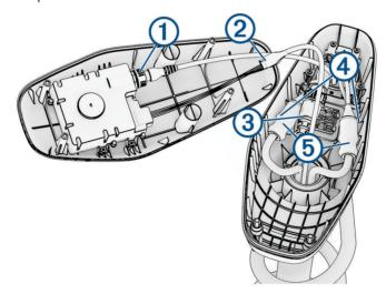
2 Release the latch 2 and pull the connectors apart to disconnect the motor data cable.
