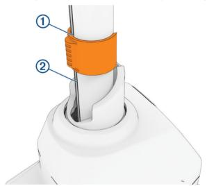
2 Slide the mini-tumbler into position in the steering servo.
