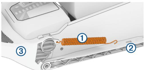
2 Repeat this procedure for the latch tension spring on the other side.
