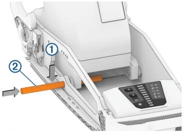
3 Push the pivot pin 2 through the mount base and the steering servo.
