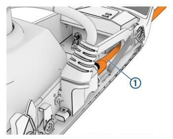
**TIP:** If you are routing a transducer cable and a power cable, you should route the transducer cable first to prevent snagging.
