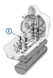
When replacing the transducer, you should dispose of the six screws. New screws, washers, and bushings are provided in the transducer replacement kit.
