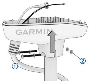
You should keep these bolts and nuts in a safe place, because you must use them when reinstalling the shaft cap.
