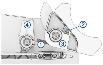
2 Secure the hook on the cradle tension spring to the notch on the cradle hook 4.
