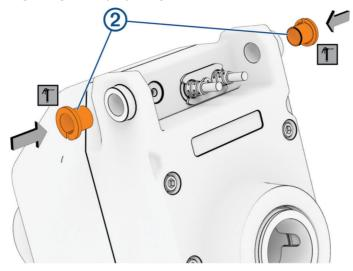
4 Insert the bushings into the steering servo housing.
