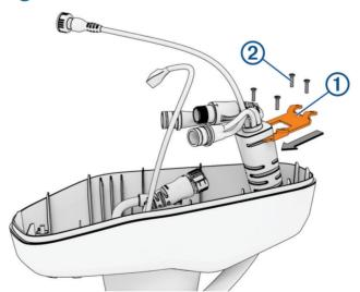
3 Secure the coil cable bracket to the shaft cap with the screws you removed earlier 2.
