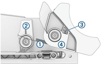
2 Using a small flathead screwdriver or a pick, slide the loop on the end of the cradle tension spring 3 off of the hook inside the cradle catch 4.
