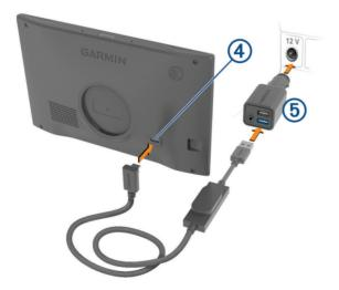
4 Plug the other end of the vehicle power cable into the vehicle power adapter 5.
