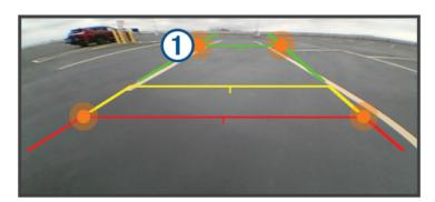
4 If necessary, reposition the vehicle with the other side closely aligned to a curb, driveway, or parking stall lines, and repeat the alignment process.
