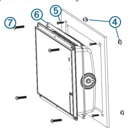
**16** Secure the nut plate to the mounting surface by fastening an included M3 screw 5 through the smaller 3.5 mm ( $^{1}/_{8}$  in.) hole.
