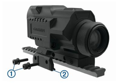
3 Tighten the screws to a maximum torque specification of 2.5 N-m (22 lbf-in.).
