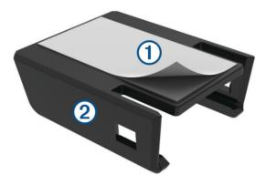
4 Press the remote trigger cable clip onto the grip of your crossbow where you can comfortably activate it while aiming.
