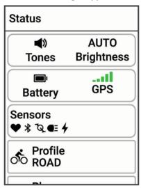
A flashing icon means the device is searching for a signal. A solid icon means the signal was found or the sensor is connected. You can select any icon to change the settings.
