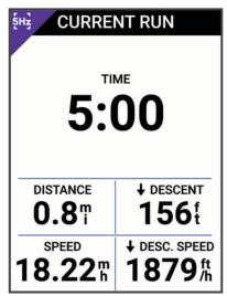
NOTE: The bike computer does not record data at 5Hz while in battery saver mode.
