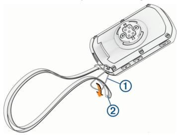
2 Thread the other end of the tether through the loop, and pull it tight.
