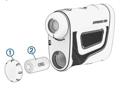
**NOTE:** You should verify the gasket and battery compartment are free of debris.
