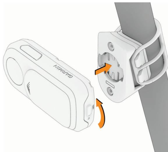
**2** Press down slightly and turn the device clockwise until it locks into place.
