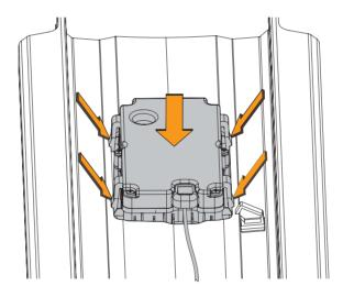
**4** Feed the cable from the replacement display panel through the upper link, taking care to feed the cable completely through the upper link.
