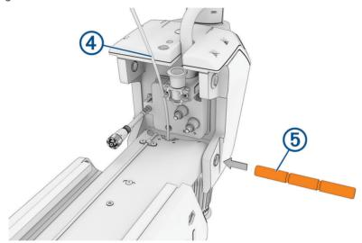
5 While lifting up on the steering system, push the pivot pin (5) through the housing and the link to hold it in place.
