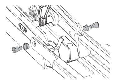
**TIP:** The bolts that secure the upper link to the mount base are fastened very securely at the factory. You may need to use a ratchet to hold the 8 mm hex bit to provide the leverage needed to loosen these bolts.
