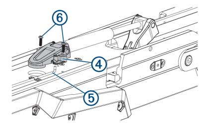
7 Using a #2 Phillips screwdriver, install the two screws 6 that secure the lower gas spring clevis to the lower link of the mount.
