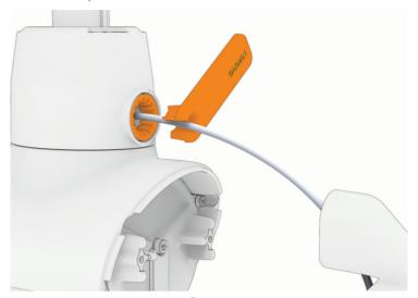
2 Carefully pull the transducer cable straight down 1 through the bottom of the shaft until it is completely removed from the shaft.
