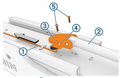
2 If necessary, pivot the upper gas spring 2 toward the lower link of the mount so the base of the gas spring aligns with the safety rod and mounting holes.
