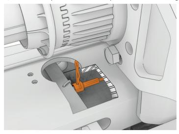
3 Remove the end of the pull cable through the access hole, and pull to remove the rest of the cable from the steering system housing.
