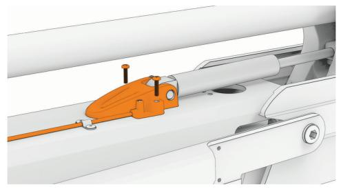
3 Lift the lower gas spring clevis off of the safety rod.
