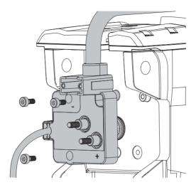
2 Pull the coil cable block away from the steering system to remove it.
