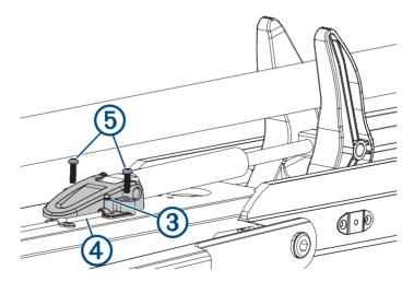
7 Using a #2 Phillips screwdriver, install the screws (5) that secure the lower gas spring clevis to the lower link of the mount.
