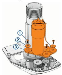
4 Lift up and remove the steering servo motor from the housing.
