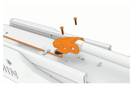
2 Lift the upper gas spring clevis off of the safety rod.
