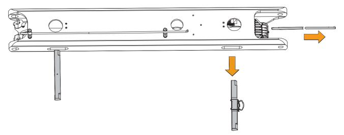
4 Slide the two latch bars out of the lower link.
