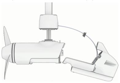
3 Holding the cables only, slowly pull them out of the shaft, taking care that the cable connectors do not get caught on the top of the shaft.
