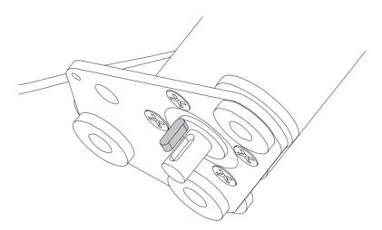
5 Remove the shaft carrier 4, the drive gear 5 and the steering position sensor gear 6 and set them aside.
