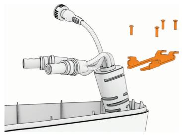
2 Pull the coil cable out of the shaft cap to remove it.
