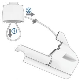
3 After you pull the transducer cable through the shaft completely, pull it through the hole in the front of the shaft base 2, along with the cable gland.
