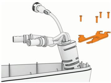
3 Secure the coil cable bracket to the shaft cap with the screws you removed earlier.
