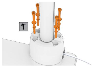
13 Using the grease packet included in the shaft and motor hardware service kit, apply grease to the 4.75 mm ( $^{3}/_{16}$  in.) O-ring on each bolt.
