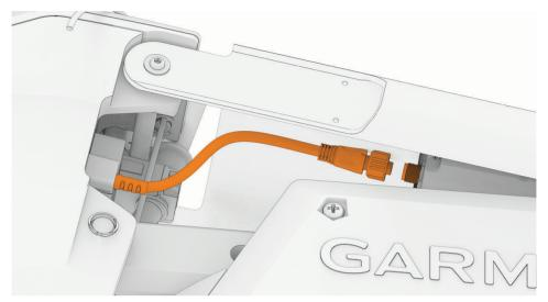
2 Using a 4 mm hex bit or wrench, remove a screw and washer from one side of the upper pin on the steering system.
