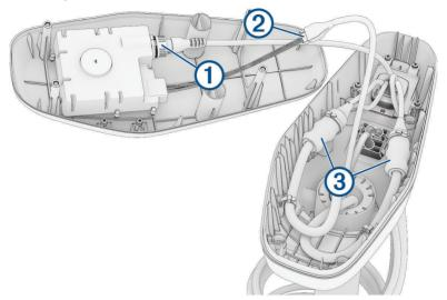
3 Release the latch and pull the connectors apart to disconnect the motor data cable 2.
