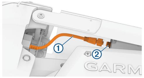
2 Push the connector onto the port on the display panel, and rotate the locking ring clockwise to secure it.
