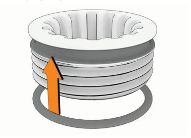
2 With the O-ring facing the transducer, feed the transducer cable through the recessed nut and the hole in the front of the shaft base 1, but do not feed the cable up through the shaft.
