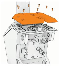
2 Lift up and remove the electronics cover.
