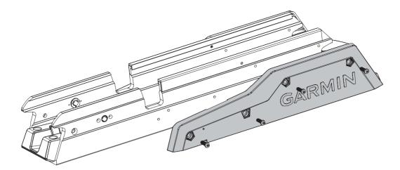
2 Secure the replacement shrouds to the mount base using the screws provided with the replacement shrouds.
