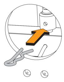
**TIP:** You can use needle-nose pliers to push the R-pin, if necessary.
