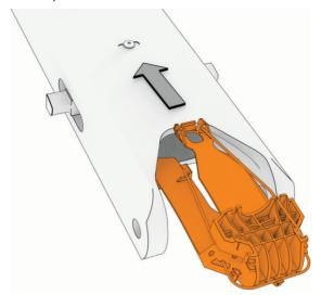
2 Make sure the bushings in the mount base are present. If necessary, insert them from the inside.
