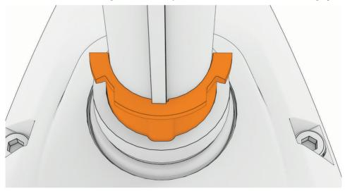
5 Install the smooth bushing over the other side of the shaft and slide it down until its lip rests on the steering system housing.
