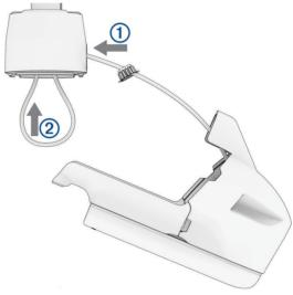
3 Leaving about 60 cm (2 ft.) of the transducer cable out of the front of the shaft base, feed the transducer cable up through the shaft ②.
