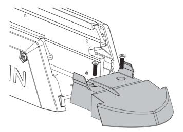
2 Install the replacement mount bumper, and secure it to the mount base using the screws provided with the replacement part.
