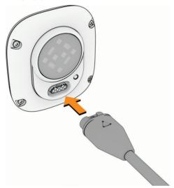
3 Plug the other end of the cable into a USB charging port.
