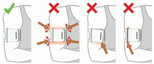
Position the module pocket and retaining bar on the outside of the arm, so that the module faces out.
