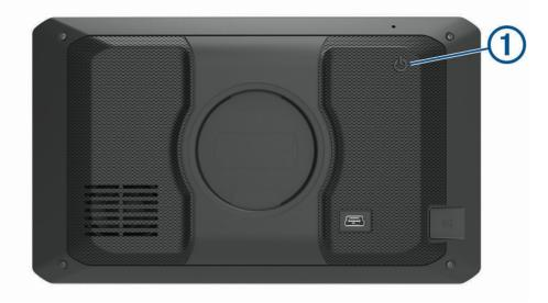
To put the device in power saving mode, press the power key while the device is on.
