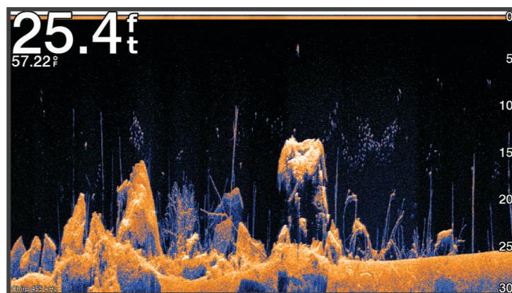
Traditional transducers emit a conical beam. The Garmin ClearVü scanning sonar technology emits a beam similar to the shape of the beam in a copy machine. This beam provides a clearer, picture-like image of what is beneath the boat.
