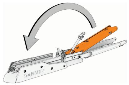
2 Push the two safety rods 1 into the lower link as far as possible.
