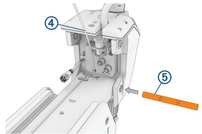
5 While lifting up on the steering servo housing, push the pivot pin (5) through the housing and the link to hold it in place.
