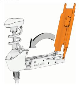
4 Tip the top of the steering servo housing inward so the holes on the upper link and the housing align.
