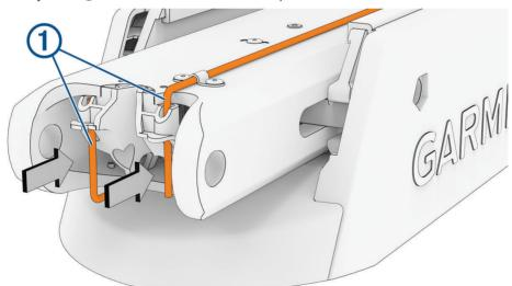
3 Make sure that the bushings 2 are installed in the lower holes 3 on the steering servo housing.
