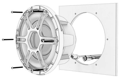
17 Secure the subwoofer to the mounting surface using the included screws.
