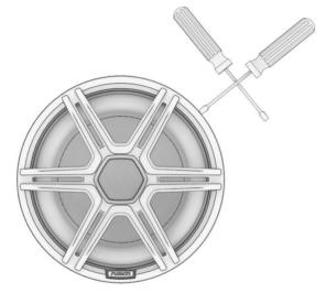
**NOTE:** For the best results, avoid placing the prying tool in the middle of a retention tab. The grille is easier to remove when starting at either edge of a retention tab.
