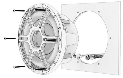
**17** Secure the subwoofer to the mounting surface using the included screws. **NOTE:** Do not over tighten the screws.
