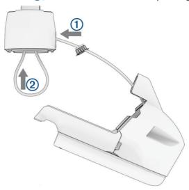
**5** Leaving about 60 cm (2 ft.) of the transducer cable out of the front of the shaft base, feed the transducer cable up through the shaft 2.
