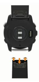
**NOTE:** Make sure the band is secure. The latch should close over the watch pin.
