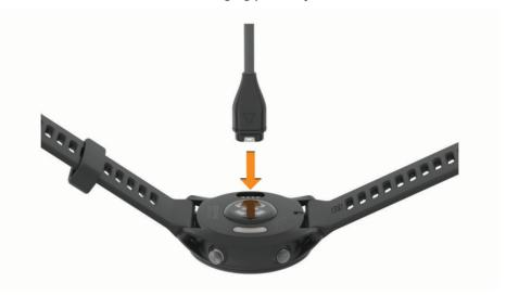
2 Plug the large end of the USB cable into a USB charging port. The watch displays the current battery charge level.
