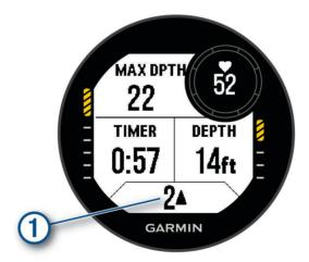
**In-dive screen**: Displays the information about the current dive, including the elapsed time, current and maximum depth, heart rate data, and rate ascent or descent. You can edit three of the data fields (*Customizing the Data Screens*, page 41).
