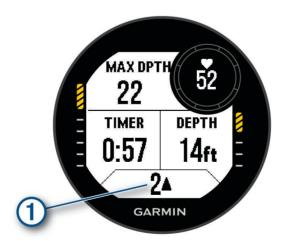
**In-dive screen**: Displays the information about the current dive, including the elapsed time, current and maximum depth, heart rate data, and rate of ascent or descent. You can edit three of the data fields (*Customizing the Data Screens*, page 41).
