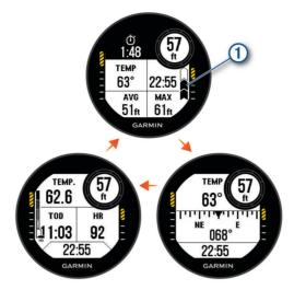
**Dive stopwatch**: Displays the bottom time stopwatch, average depth, maximum depth, and rate of ascent (*Using the Gauge Dive Stopwatch*, page 17).
