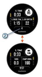
**Surface interval screen**: Displays the current surface interval time, as well as the elapsed time, maximum depth, and temperature for your last apnea dive. You can edit the data fields.
