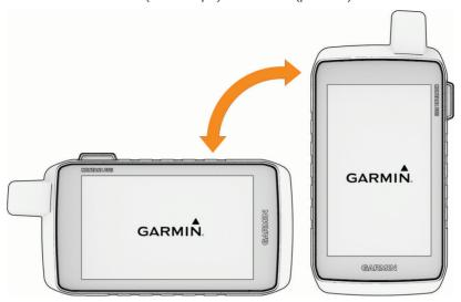
**NOTE:** While using the inReach features of your Montana 700i/710i/750i/760i device, you should use the device in vertical (portrait) mode, with the antenna pointed toward the sky.
