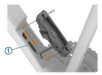
**NOTE:** Avoid touching or moving the O-ring ① to ensure the cables connect and seal correctly.
