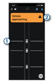
The vehicle position ① moves up the screen as a vehicle gets closer to your bike. The threat level banner ② changes color based on the potential level of threat. Green indicates no vehicle is detected. Amber indicates a vehicle is approaching. Red indicates a vehicle is advancing at a high rate of speed.
