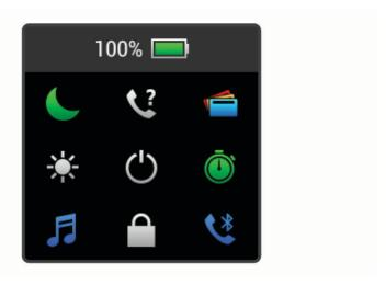
The controls menu contains customizable shortcuts, such as locking the touchscreen and turning the watch off. **NOTE**: You can add, reorder, and remove the shortcuts in the controls menu (*Customizing the Controls Menu*, page 38).
