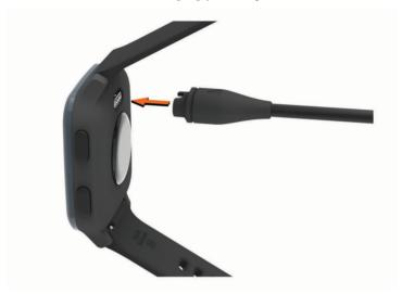
2 Plug the large end of the USB cable into a USB charging port. The watch displays the current battery charge level.
