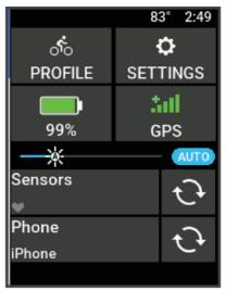
The settings widget appears. A flashing icon means the device is searching for a signal. A solid icon means the signal was found or the sensor is connected. You can select any icon to change the settings.
