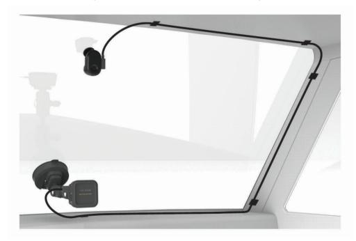
The cable is designed to be routed out of sight. To hide the cable, route it behind the vehicle trim along the windscreen, doorframe or dashboard.
