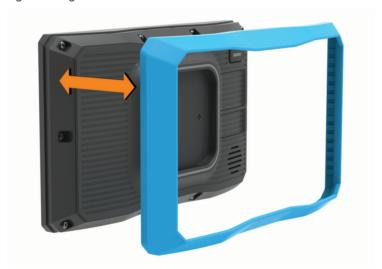
3 Place the new trim ring on the device and snap it into place.
