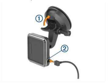
2 Plug the vehicle power cable into the port (2) on the mount.
