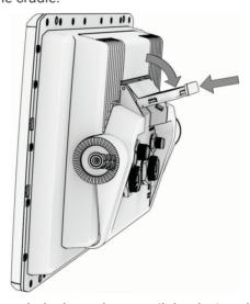
5 Press the button on the lever, and push the lever down until the device clicks in place.
