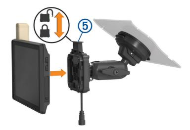
9 Push down the lock 5 to secure the device to the mount.
