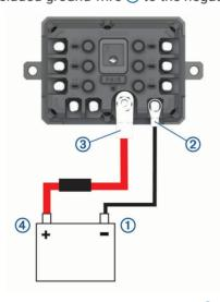
2 Connect the small ring end of the ground wire to the GND terminal 2 on the device.
