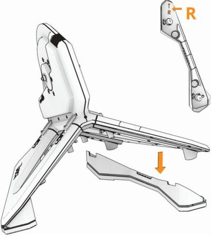
5 Check the alignment of the plates on both sides.You may need to lift and adjust each side to align the plates correctly.NOTE: Both plates must be fully seated.
