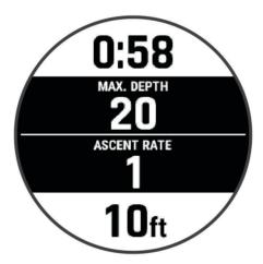
**In-dive screen**: Displays the information about the current dive, including the elapsed time, current and maximum depth, and rate ascent or descent. You can edit the data screen layout and data fields (*Customizing the Data Screens*, page 100).
