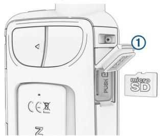
2 Insert the memory card with the gold contacts facing the front of the device.
