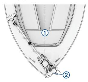
You must install the mount with the top of the cutout ② overhanging the gunwale of the boat. The U shape should extend over the side of the boat.
