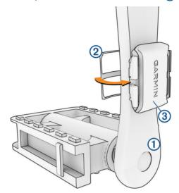
4 Rotate the crank arm to check for clearance.
