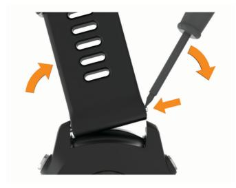
**NOTE:** Make sure the band is secure. The watch pin should align with the holes on the device.
