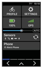
The status widget appears. A flashing icon means the device is searching for a signal. A solid icon means the signal was found or the sensor is connected. You can select any icon to change the settings.
