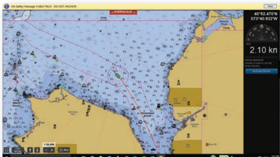
Safety message received by the vessel's electronic navigation display
